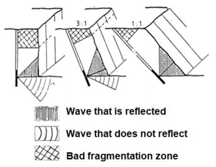
Along with the disadvantages, it is worth emphasizing the operational difficulties in using angles greater than 20°, because although in specific scenarios they can be circumvented, in large operations these difficulties can represent a great impact on the productivity and performance of the operation. Therefore, we need to consider the following points:
