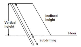
In general, both theoretical concepts and practical applications have indicated that the use of inclined holes in open-pit blasting, mainly in benches, produces better results, where the main reasons for this would be:
