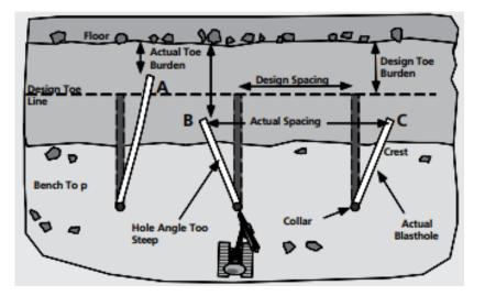
It is very important that the sloped holes are clearly oriented with proper alignment, following the slope of the free face or more precisely the material release direction.
