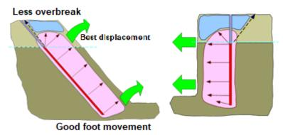
Another point that we need to be very attentive to when using inclined holes is their alignment (direction), as a wrong alignment will eliminate any advantage of the inclination, and most of the time will create a scenario of losses much greater than any potential benefit. That's why it's important to be mindful of the fact that angled holes require an accurate and reliable drill alignment system to ensure the hole is going in the right direction.
