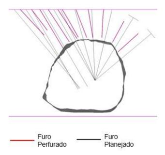
Figure 14: Execution of holes with an angle and length different from the Project.
