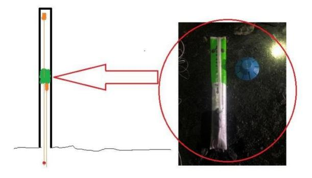
Figure 11: Illustration of deck loading and use of air pockets as separators.
