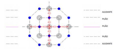
Figure 4: Slot drilling plan with relief and production holes.
