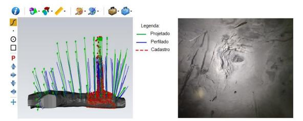
Figure 13: Topographic registration performed with scanner and photo after blast.
