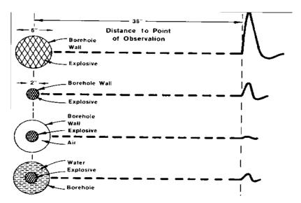
Then we have a small diameter hole, but still completely engaged, and we see that the decrease in the peak pressure is directly due to the reduction of the explosive charge.
