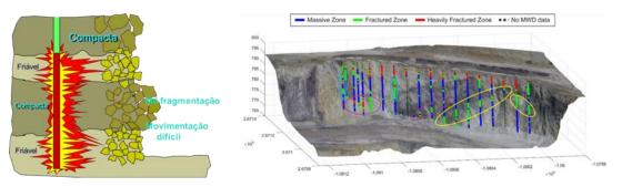
An important detail regarding the characteristics of the rock, is that the fragmentation process is much more efficient in compact and homogeneous rocks, because as we have fractures, discontinuities, or changes in rock properties, we will have a greater interference in the process of fragmentation, usually resulting in lower efficiency.
