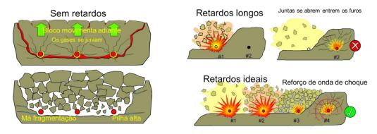
Another point of view, which is also widely accepted, and which the time intervals practically coincide, is to consider that the second hole must detonate when the shock waves from the first hole reach it, so that, when detonating, the shock waves will have a maximum interaction in the area of the second hole.
