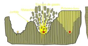
When the fractures are in the same alignment as the holes, they can direct the energy of the hole that is detonated first to the other hole, and thus it can initiate it out of sympathy, or even desensitize that hole, and this will impact the result of our blast.
