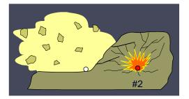
In summary, we can say that when we detonate several holes instantly, or with a very short interval of time between them, we will have a very strong initial performance of the pressure, but it is quickly relieved, generating a strong frontal launch, but the performance quick release of pressure, does not cause effective fragmentation.
