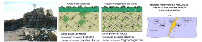
Usually the discontinuities will negatively impact the process, limiting the propagation of fractures, causing disturbances in the interactions between waves, and also decreasing the pressure of the gases, due to the greater empty space available, in the same way as they can create points of weakness, which allow the gases escape, further decreasing its efficiency.
