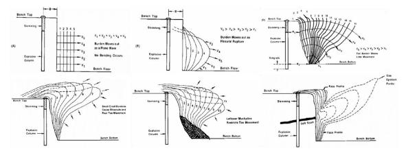
We can see in each example, that as we have anomalies on the free face, whether in a punctual way, or along the face, we will have a disturbance in the expansion of gases, and this will affect the release of the material, and in the same way, the process of fragmentation.
