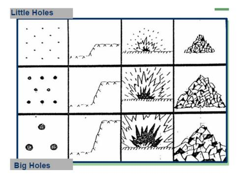
The other parameters of the hole, such as depth, inclination and sub-drilling also influence the fragmentation process, mainly with regard to the effect of rock bending and the interaction between the holes.
