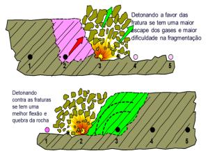
greater bending of the rock. Also, when necessary, increase the burden to hinder the escape of gases, and decrease the spacing to increase the interaction between the holes..
