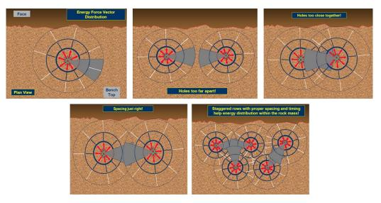
Still with regard to the mesh, the spacing between the holes in the same line will influence the level of interaction between the holes, while the spacing will interfere more with the reflection of the waves.
