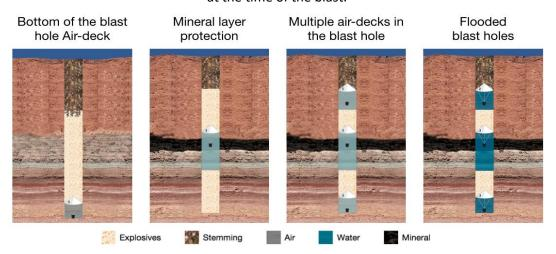
The ideal would be to have the energy of the explosive acting perfectly and the same at all points of the rock, but this does not happen, because the distribution of the explosive, and of the energy generated in its blast, is not uniform within the rock mass, and will directly depend on the configuration of our explosive charge, as well as the operational quality in carrying out the proposed charge configuration.
