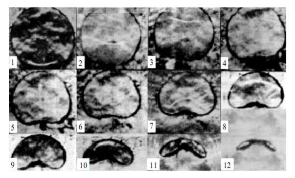
And as we said, at this moment in frame 12, when the bubble is compressed to its maximum, we have an increase in pressure and temperature to the point that it cannot withstand it and that is when it will burst, generating a shock wave, caused by the rapid expansion of the gas inside the bubble.
