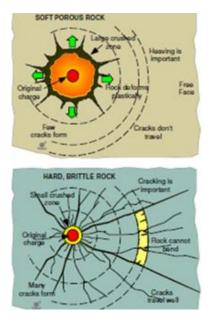
The first fragmentation zone, in the region surrounding the hole, is responsible for most of the fine material produced by the blast, but it represents a very small portion of the rock, so when the objective of fragmentation is to seek a greater amount of fines, it is necessary to maximize this zone as much as possible during the blast, looking for explosives that generate a greater initial shock wave, and also using a greater number of holes.
