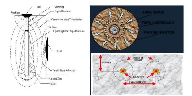
When the shock wave arrives at the free face, it is reflected on this surface, returning to the interior of the rock, and now making an opposite pressure effort, in front of the waves that continue to compress the rock, it generates traction and shear forces in the rock, which normally has a much lower resistance to this type of effort, and so we begin our second phase of the fragmentation process.
