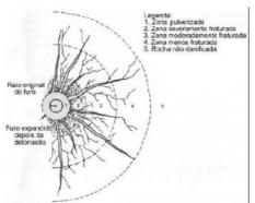
their maximum expansion, and thus causing a great bending in the rock, and when it exceeds its limit, the gases break through the rock completely, and are dispersed into the atmosphere.
