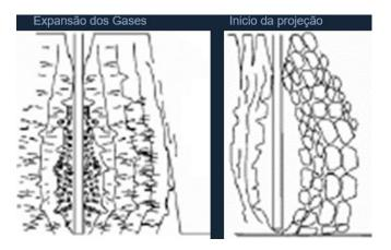
Following this reasoning, we have that the effect caused by the gases in the rock, is generated by the pressure that the gases exert on the walls of the hole during the blast of the explosives, and this pressure generated by the gases will be related to the total volume of gases and the great increase the temperature of these gases.
