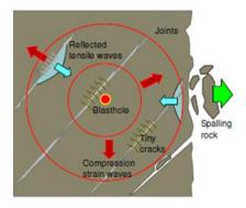
This has two sides, on the one hand, it contributes to the application of fractures and the creation of new fractures, helping in the fragmentation process, but on the other hand, if these fractures are very representative and with large extensions, many waves will be reflected in them, opening them up. as, and this can cause the gases, which are starting to penetrate the fractures, to find exits from the rock, losing intensity.
