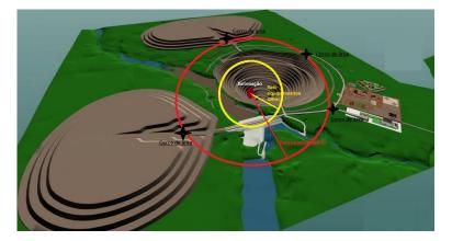
That's why we usually focus much more on concepts related to the open pit environment, as it is much more extensive and has a much greater radius of influence, in addition to the fact that open pit blasts are usually much larger than underground blasts, and that clearance zone concepts are easily adaptable to either environment.
