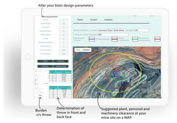
The software works directly through an online platform and has a mobile application for cell phones, which can be easily used in the field, allowing us to change the data and visualize the danger zones for equipment and people on the operation map, where in any situation critique, we can change the parameters of the blast plan on the spot and immediately assess the reflection at the boundaries of the areas.
