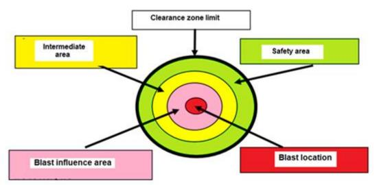
First, we have in our figure, our central point, represented here in red, which indicates the blast location, that is the place where we will perform our blast, and represents the volume or block rock in which we will be applying the explosives to carry out the rock blasting process.
