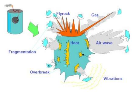
Below we have an example (Berta) of the distribution of the energy consumed in the blasting process for a rock blast:
