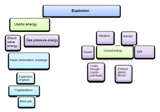
Just below we have an illustration of the distribution of energy spent in the blast process:
