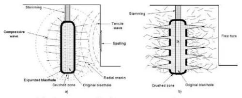
a) Shock wave propagation, b) gas pressure expansion
