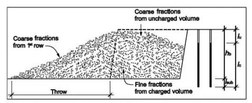
Typical profile through a rock pile from a surface blast, indicating the main fragmentation sections
