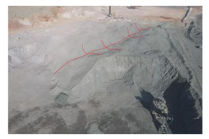
This detonation has already managed to use electronic detonators and carry out a more adequate design in the contact region, which facilitated the design of the timing, but due to the limitation of the free face, it was not possible to direct the material to opposite areas.
