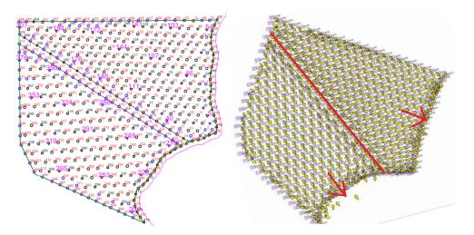
Two very important points that we could see in this detonation were first that the free face limitation had a direct impact on the size of the "separation valley", because without enough space the material blistered upwards, limiting the separation, and the second was a ratio reduction of load used due to the low DF of the drills decreased the launching force, which limited the separation of the materials, but contributed to the preservation of the contact of the materials.
