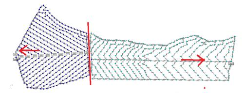
As the areas had very different shapes and dimensions, including the mesh and number of holes, we started carrying out the design/timing at the contact limit, to ensure that the contact holes came out at the same time, then we determined the necessary relief for the nearby holes this region and from there we carry out the sequencing of the other holes following the standard mine design configurations.
