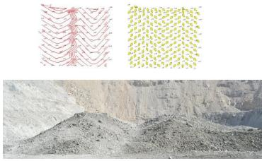
2. Preservation (Do not mix): when, during detonation, one seeks to maintain the natural conditions of contact, without the material mixing, that is, leaving them in the same original configuration after dismantling, with no or minimal movement during the detonation.
