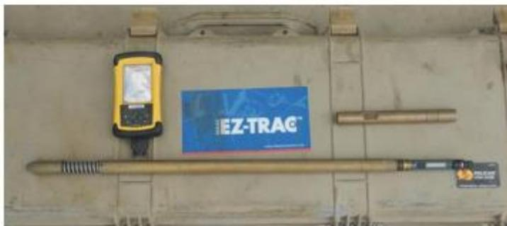
Figure 6: Survey equipment: Palmtop, Reflex Case and Rod Set
