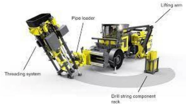
Figure 1: Easer L for relief holes
