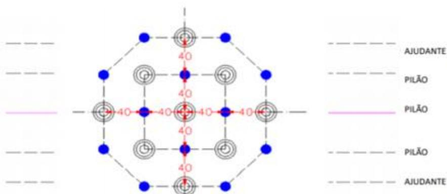
Figure 4: Slot drilling plan with relief and production holes.
