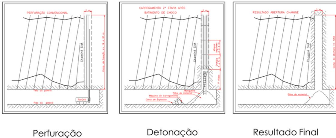
Figure 3: Steps in the blind free face opening process.
