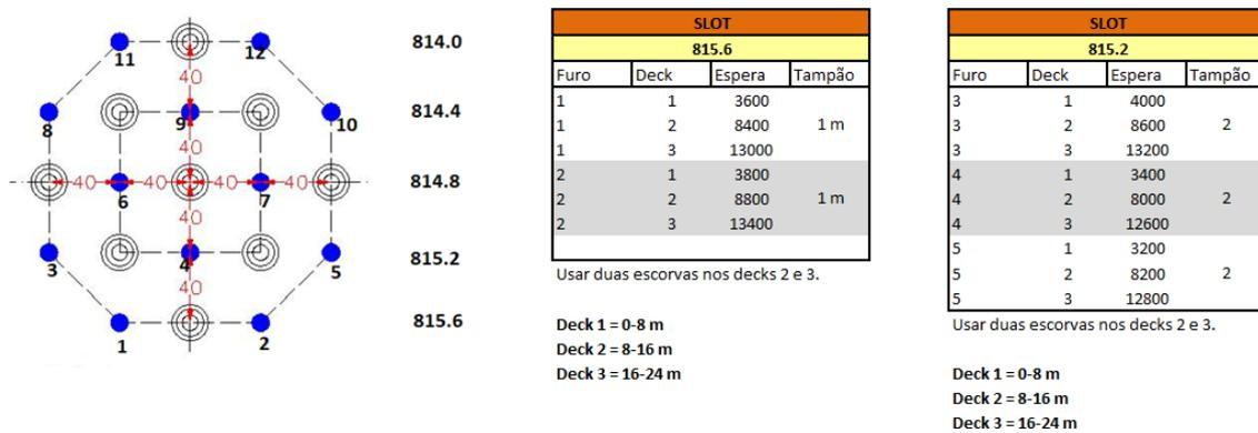
Figure 12: Timing used on each deck according to the drilling plan.
