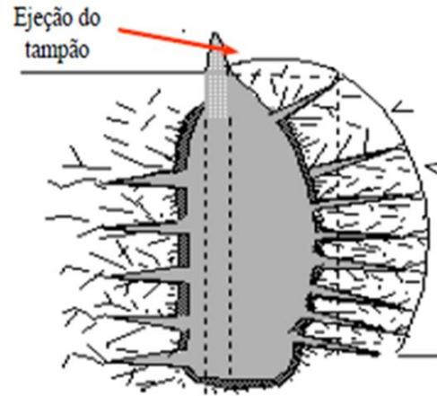
That is, we need the maximum of the energy of the explosive to be spent on breaking the rock internally, before the rest of the energy escapes, or is spent on other effects, such as material release or vibrations.
