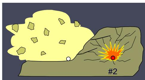
In summary, we can say that when we detonate several holes instantly, or with a very short interval of time between them, we will have a very strong initial performance of the pressure, but it is quickly relieved, generating a strong frontal launch, but the performance quick release of pressure, does not cause effective fragmentation.
