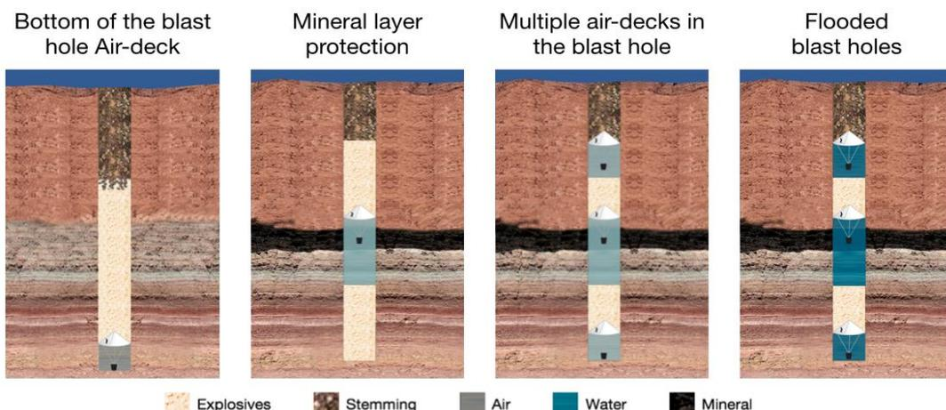
The ideal would be to have the energy of the explosive acting perfectly and the same at all points of the rock, but this does not happen, because the distribution of the explosive, and of the energy generated in its blast, is not uniform within the rock mass, and will directly depend on the configuration of our explosive charge, as well as the operational quality in carrying out the proposed charge configuration.
