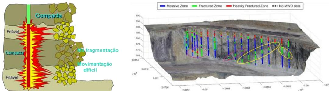
An important detail regarding the characteristics of the rock, is that the fragmentation process is much more efficient in compact and homogeneous rocks, because as we have fractures, discontinuities, or changes in rock properties, we will have a greater interference in the process of fragmentation, usually resulting in lower efficiency.
