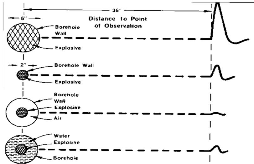
Then we have a small diameter hole, but still completely engaged, and we see that the decrease in the peak pressure is directly due to the reduction of the explosive charge.
