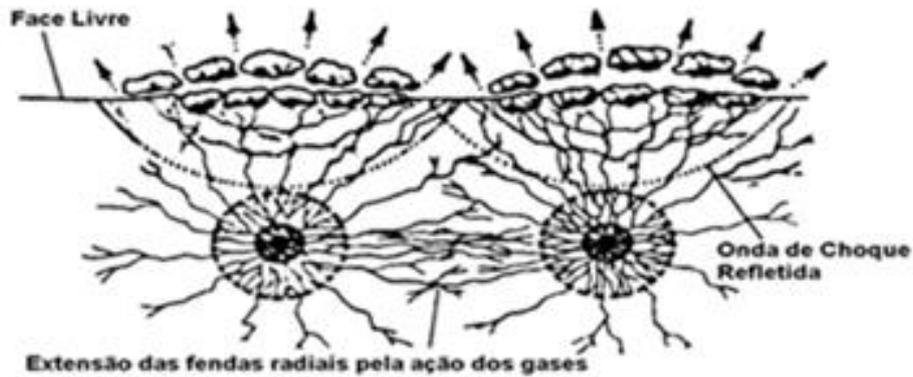
While these mechanisms are already operating in the fragmentation, the gases generated by the explosive are penetrating the fractures, extending these fractures and creating new fractures, and in the same way the shock waves that were reflected in the free face, return causing a traction effort, creating new ones. fractures and extending existing fractures.
