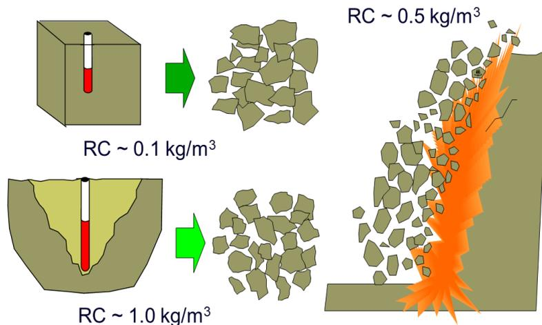
That's why most of the overbreaks we have are caused by the compressive force of the shock wave, which damages the rock as long as its intensity is greater than the compressive strength of the rock, and then just continues to generate vibrations.
