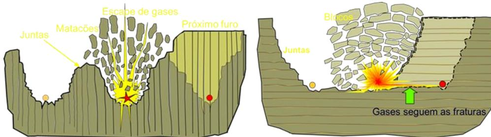
When the fractures are in the same alignment as the holes, they can direct the energy of the hole that is detonated first to the other hole, and thus it can initiate it out of sympathy, or even desensitize that hole, and this will impact the result of our blast.
