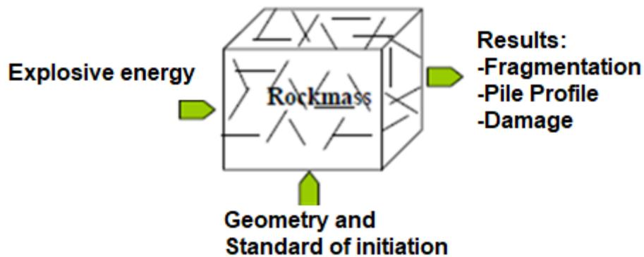
For example, we know that deviations in drilling will impact the fragmentation process, but we do not know how much this impacts, and they can even have positive and negative impacts at times, where, for example, two holes closer together should generate greater fragmentation, but they they will also be further away from their other neighbors, so fragmentation would be worse at that point.
