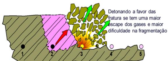
So, in cases with a large number of discontinuities, normally the standard recommendation is to sequence the holes in such a way that they detonate against the direction of the fractures, causing greater bending of the rock. Also, when necessary, increase the burden to hinder the escape of gases, and decrease the spacing to increase the interaction between the holes..
