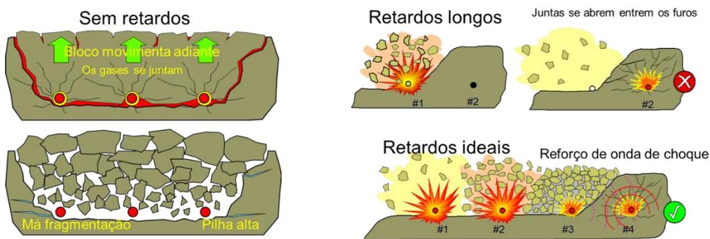
Another point of view, which is also widely accepted, and which the time intervals practically coincide, is to consider that the second hole must detonate when the shock waves from the first hole reach it, so that, when detonating, the shock waves will have a maximum interaction in the area of the second hole.
