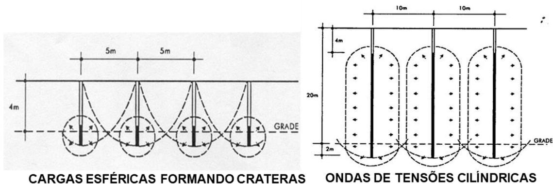
It is believed that this interaction between the different holes plays an even more fundamental role in hard rocks, as their characteristics make the interaction between the waves increase the tensile effort, and thus generate a much more intense fracturing in this type of rock. rock.
