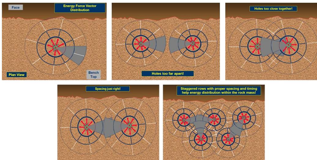
Still with regard to the mesh, the spacing between the holes in the same line will influence the level of interaction between the holes, while the spacing will interfere more with the reflection of the waves.
