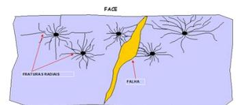
Usually the discontinuities will negatively impact the process, limiting the propagation of fractures, causing disturbances in the interactions between waves, and also decreasing the pressure of the gases, due to the greater empty space available, in the same way as they can create points of weakness, which allow the gases escape, further decreasing its efficiency.
