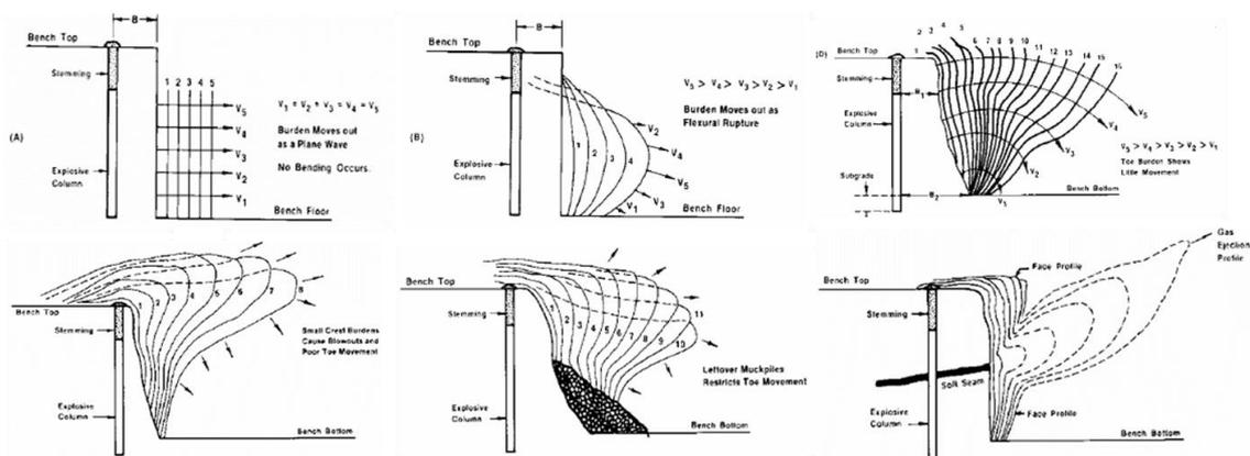
We can see in each example, that as we have anomalies on the free face, whether in a punctual way, or along the face, we will have a disturbance in the expansion of gases, and this will affect the release of the material, and in the same way, the process of fragmentation.
