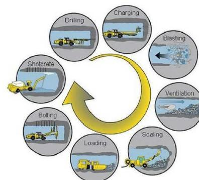
Figure 3: Typical mining drill & blast cycle
