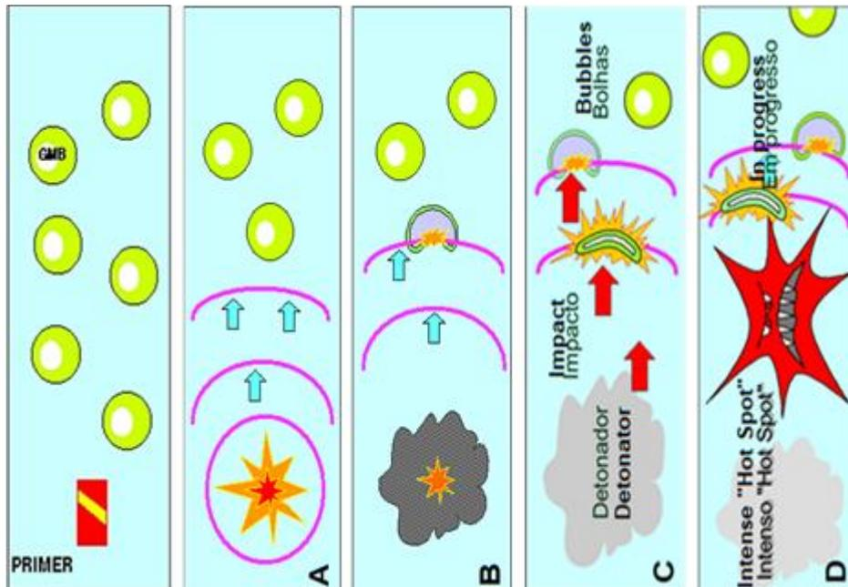
So in frame A, we have the first phase of the process, which is when the primer or initiator detonates, and with its blast, it generates the initial stimulus, which generates shock waves that will impact the explosive and start the reaction of blast
