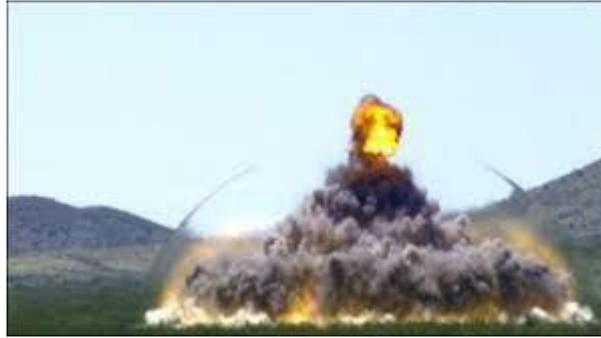
So it is common to start most theories about blast considering the explosive as a spherical and punctual charge, which releases its energy equally in all directions around it, considering that any point within the same radius would receive the same energy level and would suffer the same effects.
