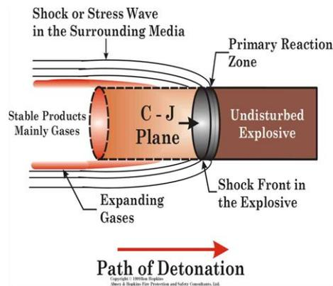
2nd) Then we have our second zone, which is the chemical reaction zone, which consists of the area where the shock wave has already passed, it is compressing the microbubbles or activating the sensitivity points, and with that some of them are breaking and others will follow soon after, continuing the process. Which we can say is represented by the gray area in our illustration on the left, also known as the “C J” plane, which is exactly where the blast reaction is taking place.
