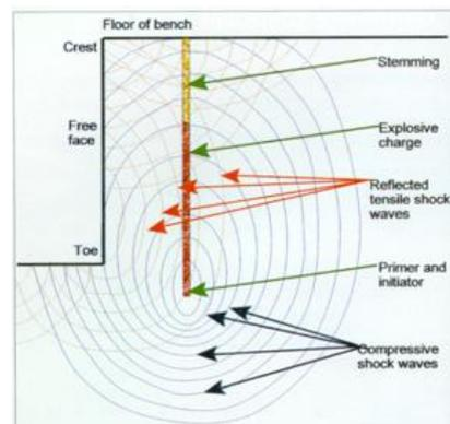
Consider that, approximately, the tensile strength of rocks is 10 to 15 times lower than their compressive strength, and therefore the effort generated by the reflected waves can cause much more intense fracturing than that generated by the waves initially .
