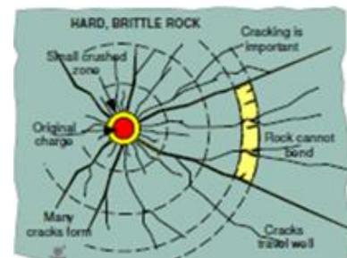
The first fragmentation zone, in the region surrounding the hole, is responsible for most of the fine material produced by the blast, but it represents a very small portion of the rock, so when the objective of fragmentation is to seek a greater amount of fines, it is necessary to maximize this zone as much as possible during the blast, looking for explosives that generate a greater initial shock wave, and also using a greater number of holes.
