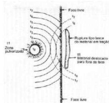
This phenomenon is even more intense when we have a spacing smaller than the ideal and a higher load ratio, as we will have a large accumulation of waves, with greater intensities, at the rock-air interface.
