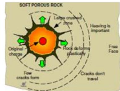
Later on, we will see that in hard rocks, the gases generated will penetrate these fractures, and any other discontinuity present in the rock, and will force these fractures to extend, increasing the level of fragmentation. Thus, the greater the number of fractures generated initially, the greater the level of final fragmentation generated in this process, influencing mainly the portion of intermediate fragments in our material.
