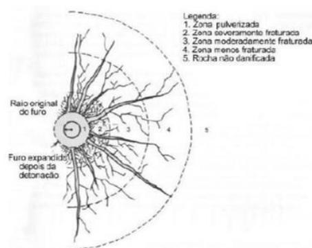
During this process, the gases continue expanding, increasing the pressure generated by this expansion, forcing the rock towards the free face, until they reach their maximum expansion, and thus causing a great bending in the rock, and when it exceeds its limit, the gases break through the rock completely, and are dispersed into the atmosphere.
