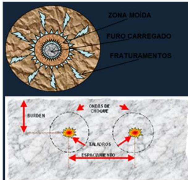
When the shock wave arrives at the free face, it is reflected on this surface, returning to the interior of the rock, and now making an opposite pressure effort, in front of the waves that continue to compress the rock, it generates traction and shear forces in the rock, which normally has a much lower resistance to this type of effort, and so we begin our second phase of the fragmentation process.
