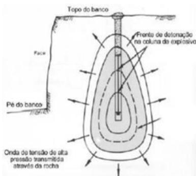
This happens because the rock's resistance to traction is much smaller than its resistance to compression, so that the wave that did not have the strength to break the rock by compression, when reflected, manages to come back breaking the rock again by an effort of traction.
