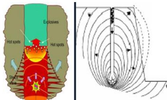
The extent of this first impact of the explosive's energy on the rock will depend on a number of factors, starting with the rock's properties, ranging from its resistance to compression, to its physical characteristics in the areas close to the hole.
