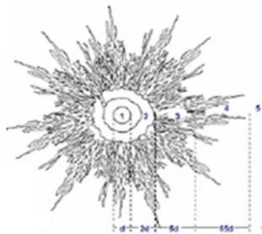
In this zone of elastic deformation, the initial shock wave no longer has the strength to exert consistent fragmentation in the rock, so its effect in this zone runs the risk of being more harmful than beneficial, as it can simply compromise the stability of the formations geological features of the rock, expanding these structures, or simply opening larger fractures, which will cause greater dissipation of gases, thus reducing the pressure generated by them at the time of their expansion.
