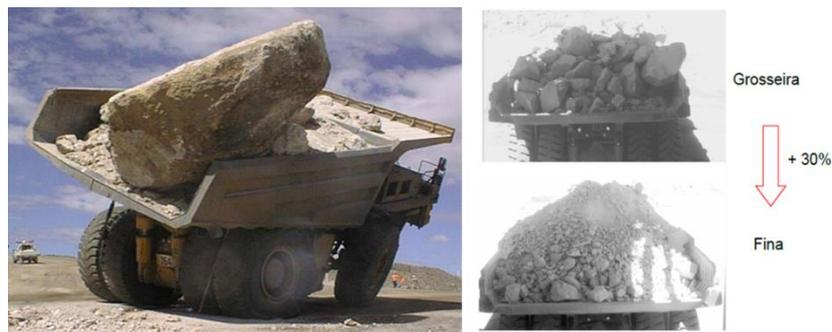
As we said earlier, our blast can also affect the floor conditions of the loading area, interfering with the maneuverability, speed and wear of loading and transport equipment.
