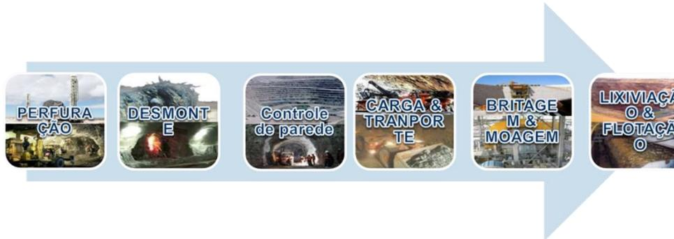
Usually the main point to optimize is the material fragmentation, as it will directly affect the crushers and mills, as well as the energy level required for the material processing.
