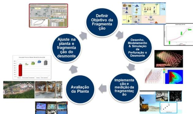
Normally in this type of methodology, the evaluation of the results of the blast is complete, where we do from indirect analysis of the productivity and efficiencies of the following activities, to a high level of control and evaluation of our blast, so that we can identify the points that need to be improved and how they affect our results.
