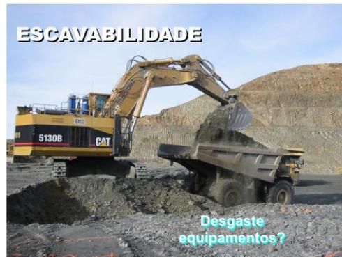
Thus, it is common to use excavator productivity as a methodology for analyzing the results of blasts, taking care to eliminate certain situations or anomalies, which may be more influenced by the operator or by the operating conditions of the equipment.
