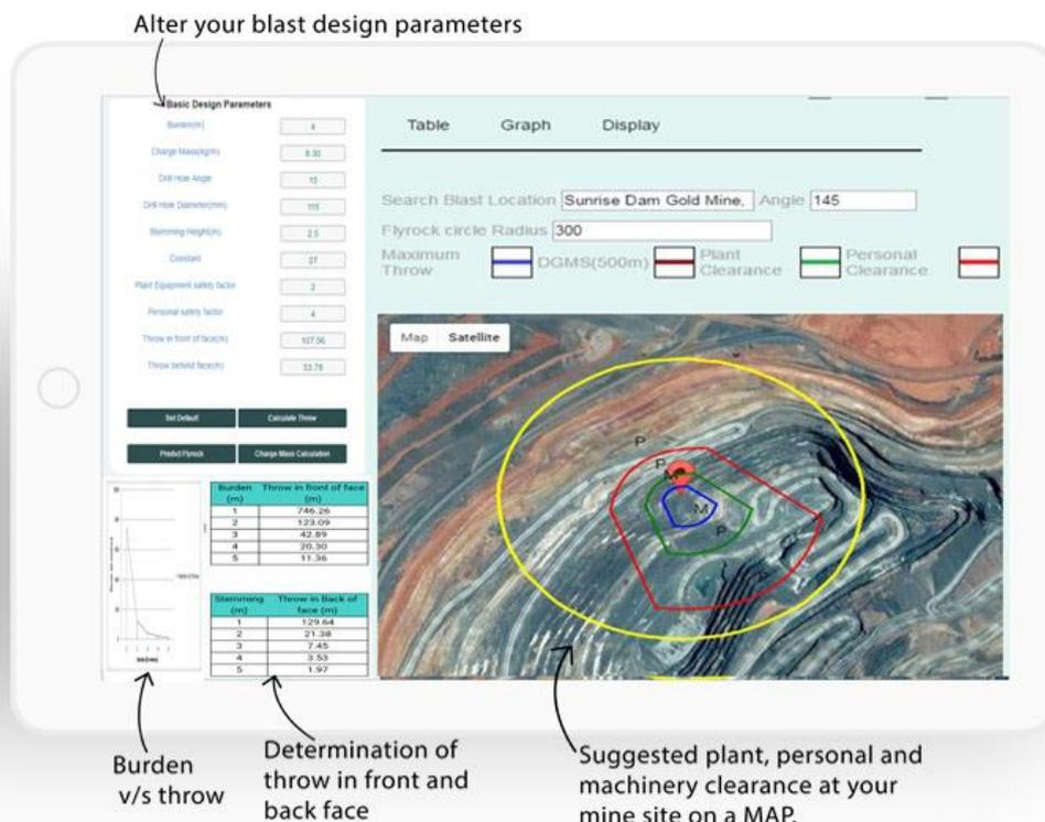
The software works directly through an online platform and has a mobile application for cell phones, which can be easily used in the field, allowing us to change the data and visualize the danger zones for equipment and people on the operation map, where in any situation critique, we can change the parameters of the blast plan on the spot and immediately assess the reflection at the boundaries of the areas.
