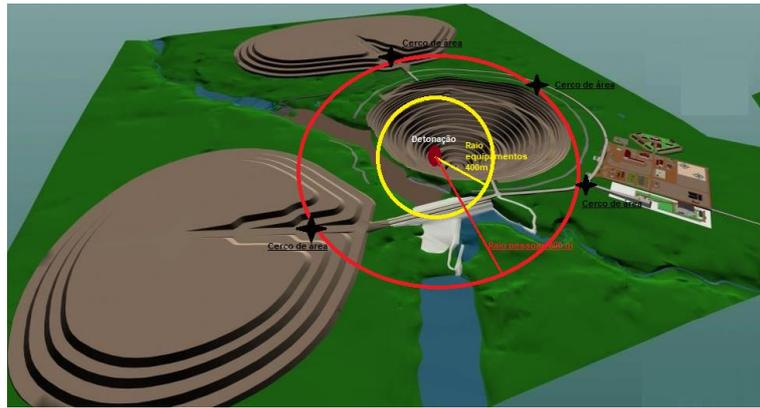
That's why we usually focus much more on concepts related to the open pit environment, as it is much more extensive and has a much greater radius of influence, in addition to the fact that open pit blasts are usually much larger than underground blasts, and that clearance zone concepts are easily adaptable to either environment.
