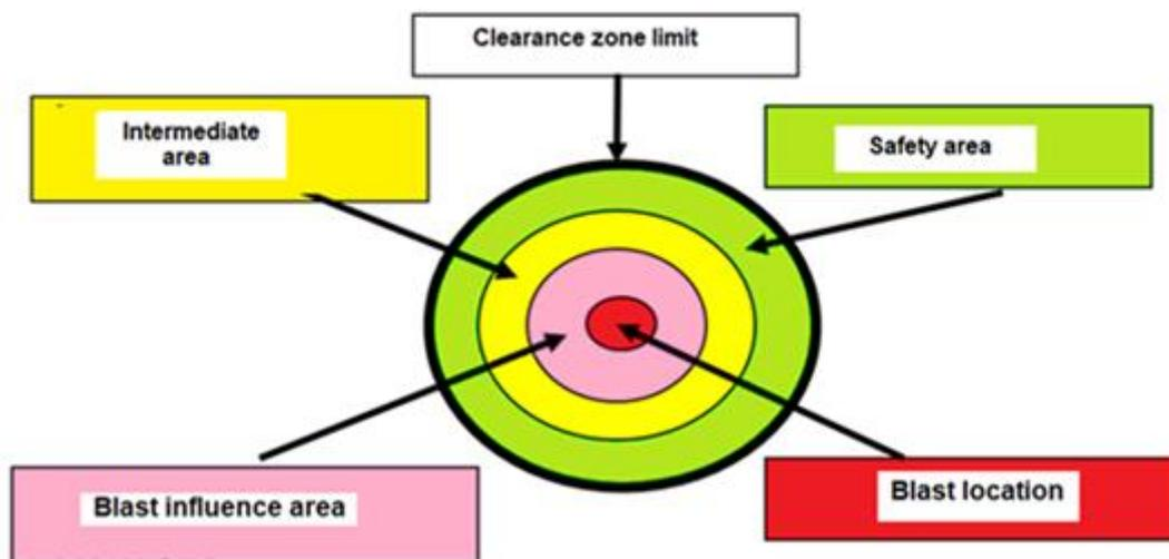
First, we have in our figure, our central point, represented here in red, which indicates the blast location, that is the place where we will perform our blast, and represents the volume or block rock in which we will be applying the explosives to carry out the rock blasting process.
